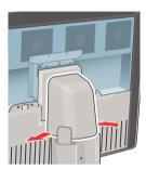
**2** Slide the cover upwards while holding the lower sides pulled open.
